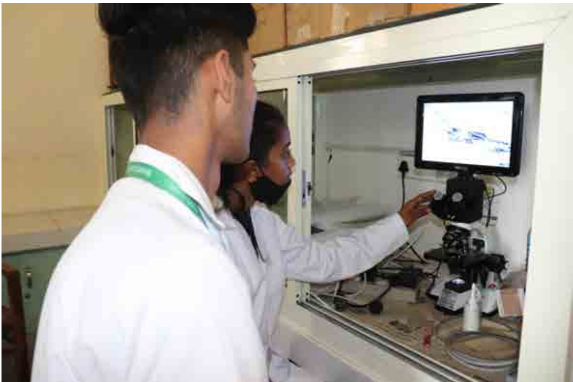
Photograph 6 Live Screen Microscope with 13.5" LED Display and Camera with provision of projection
